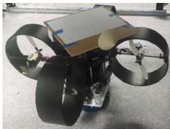
Fig. 5: Astrobees prototype 2 with VPP fans, testing on the Ames Granite Table
