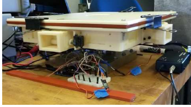
Fig. 6: Measuring centralized fan thrust performance with a two-nozzle prototype mounted on a force sensor
