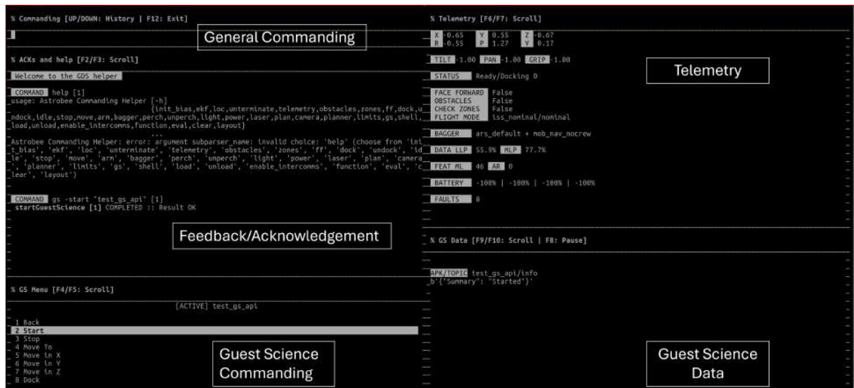
Fig. 36: GDS-Helper: Complementary text-based interface to Astrobee operators.
