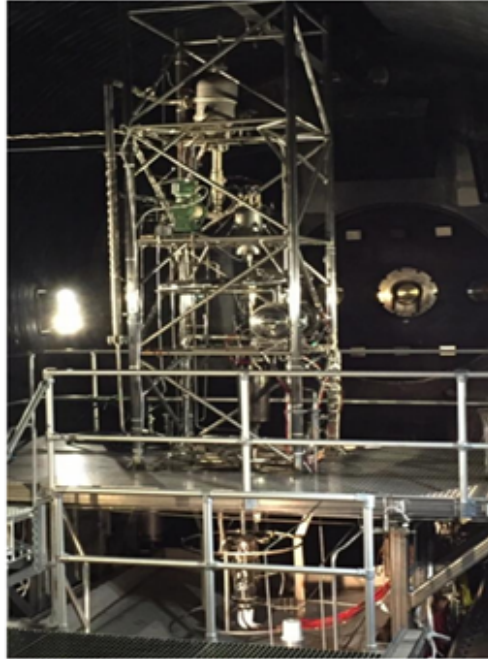
Figure 7.5: FSP TDU installed in Vacuum Facility 6 at NASA GRC.
