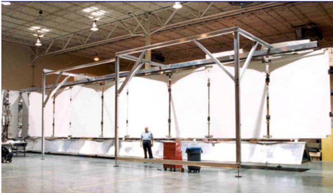
Figure 7.4: Deployed ISS pumped ammonia based PHRS panel assembly.
