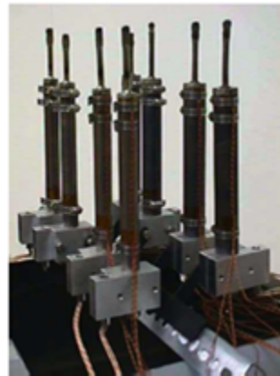
Figure 7.12: Multi-vendor HP Comparison Testing Apparatus (Project Prometheus, ref. [17, 260]).
