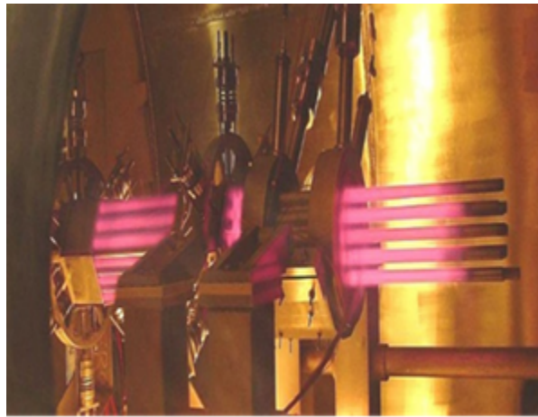
SAFE-100 1.5-cm Na Heat Pipe Testing at MSFC.
