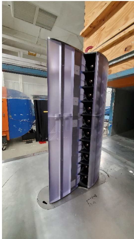
Fig. 22.—Airfoil model installed in wind tunnel facility.
