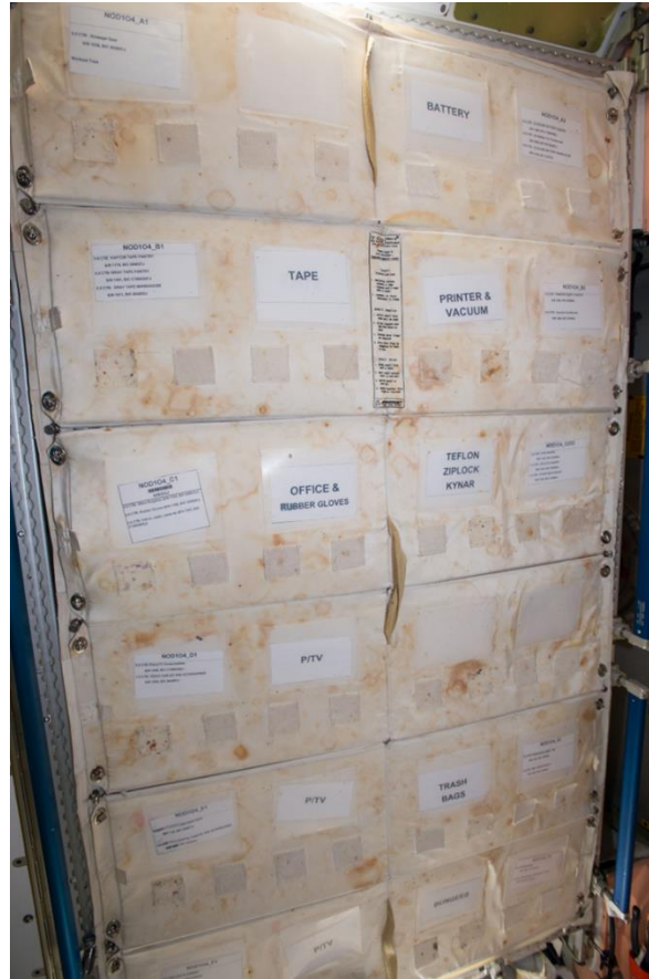
Figure 4-1. Rack in the ISS Galley Area, Stained with Food and Beverage Spills.
