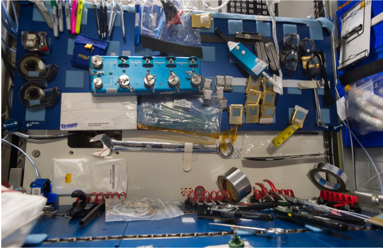
Figure 8-6. Velcro at Maintenance Work Area.
