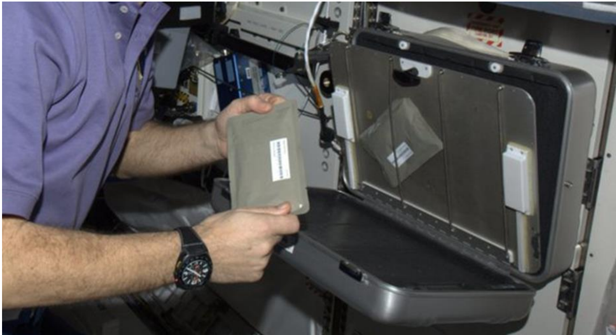
Figure 4-2. The ISS Food Warmer (AKA ISS Suitcase Food Warmer) was Portable. It could heat up to 12 ISS food/beverage packages at a time but was not deep enough to accommodate cans well. Due to the small capacity, the ISS Food Warmer was often unable to close completely when cans were being heated. Packages could be heated on both sides of the single heating plate.
