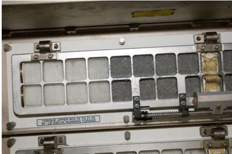
Figure 5-1. Cabin Air Bacteria Filter Assembly Before (right) and After (left) Cleaning.
