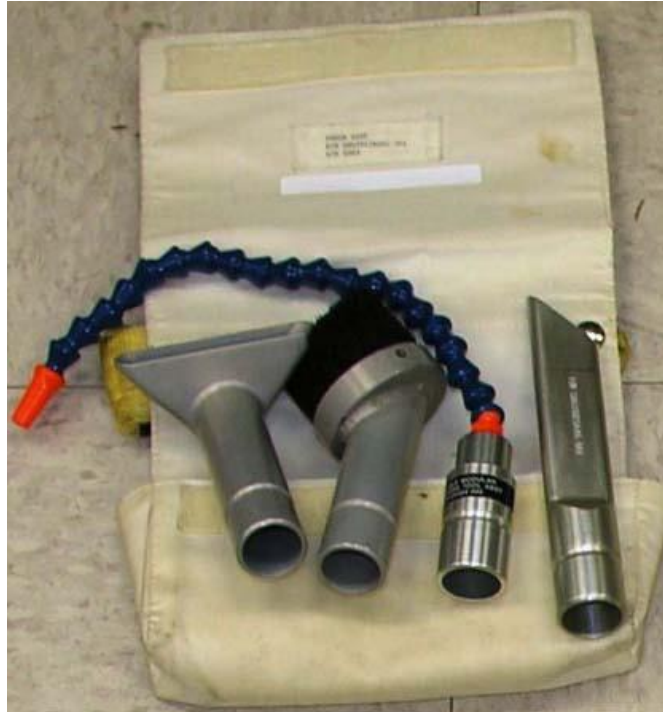
Figure 5-2. ISS Vacuum Cleaner. (Left to right): surface tool, brush tool, flexible modular cleaning tool, crevice tool.
