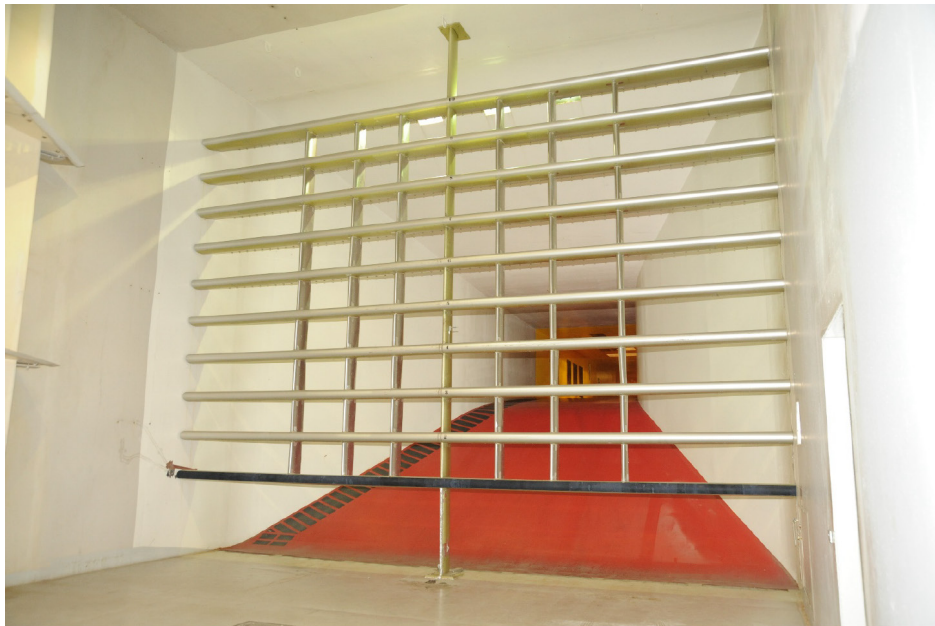
Figure 5.—Downstream view of test section through IRT spray bars.
