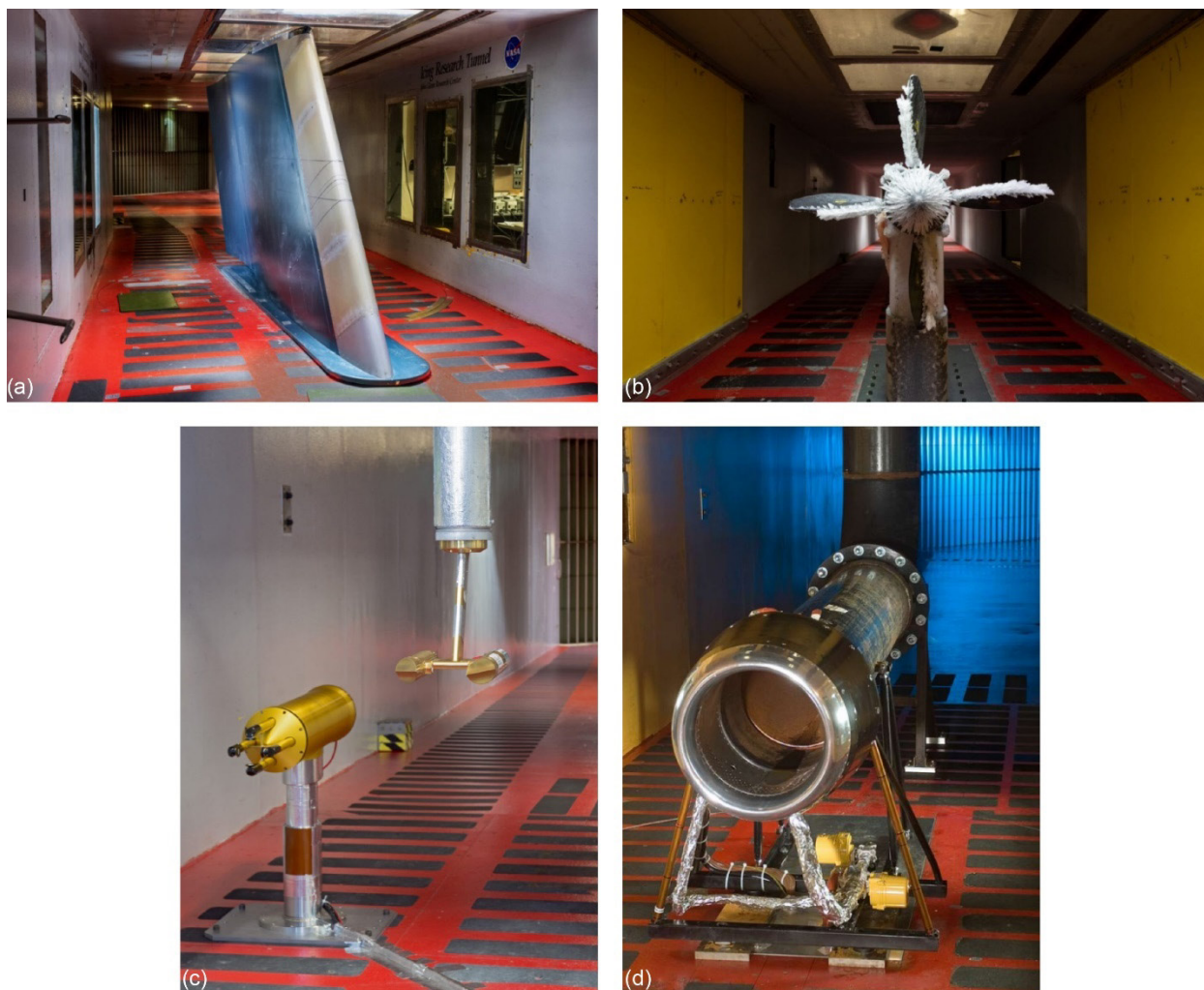
Figure 3.—Aircraft models and experiments installed in IRT test section. (a) Wing section. (b) Rotorcraft. (c) Icing instruments. (3) Engine inlet.
