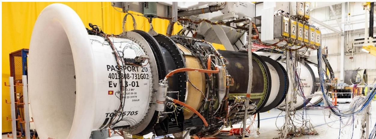
Figure 8: Final Hybrid Electric Turboman Engine Assembly
