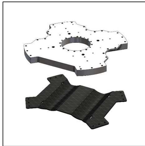
Figure 61: Electronics Deck and Substructure Support Comparison
