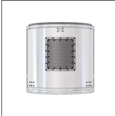
Figure 62: Skin Assembly Door and Doubler
