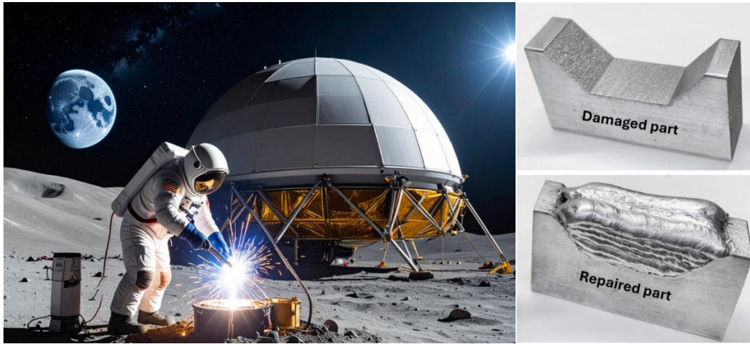
Figure 1. In-space welding used for repairing a damaged metal cavity.
