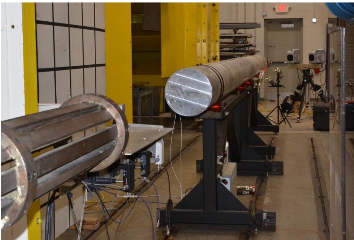
Figure 2.—Location of Hopkinson bar (center) relative to tapered section of gun barrel (left).
