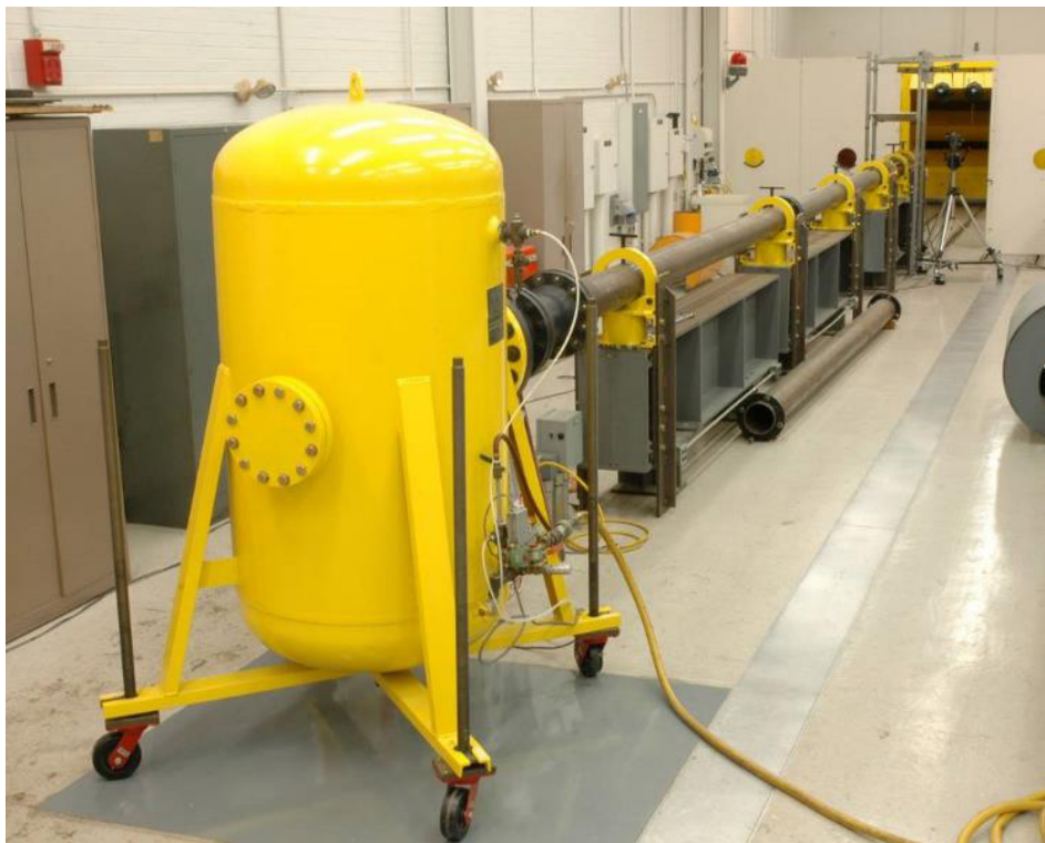
Figure 1.—Gas gun used for launching projectiles.
