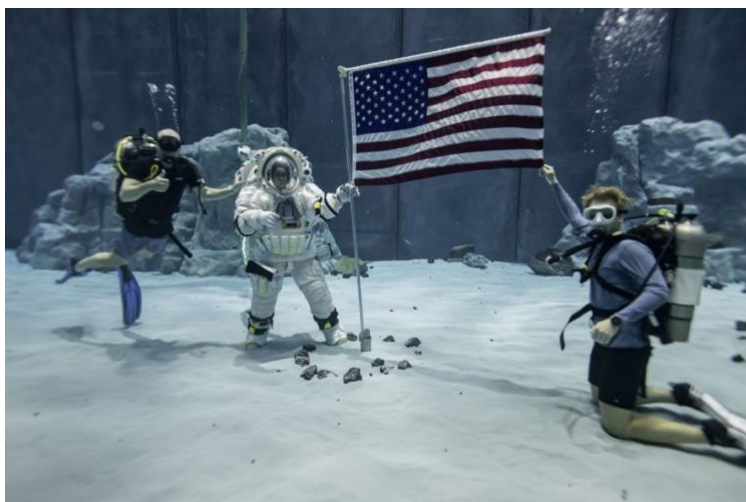
Figure 2. Engineers test lunar spacesuits being developed by Axiom Space in the Neutral Buoyancy Laboratory at NASA's Johnson Space Center in Houston [14].
