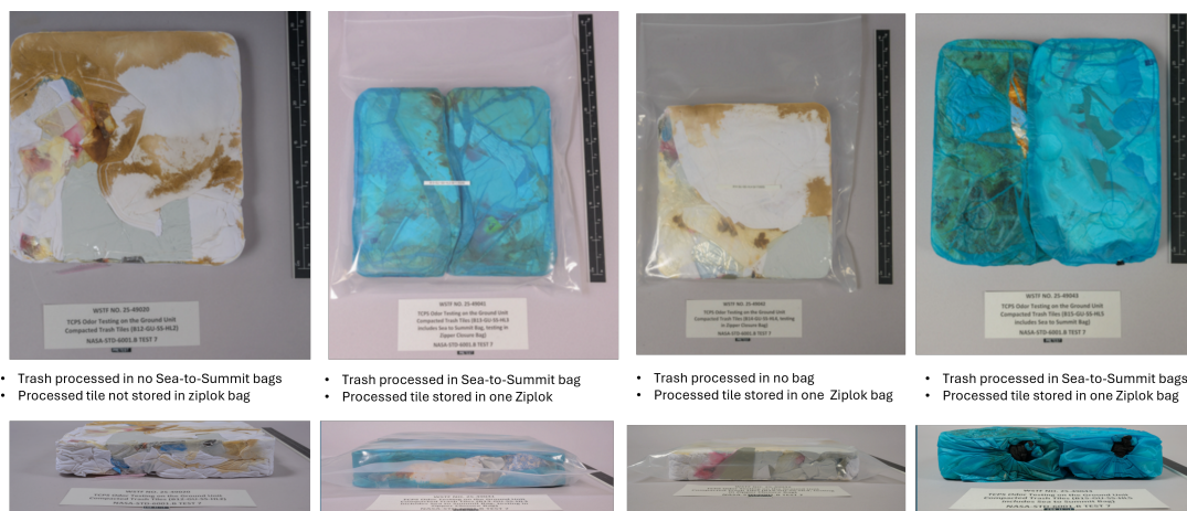
Fig. 3 Pictures of the high liquids processed tiles sent to WSTF for odor analysis[12]
