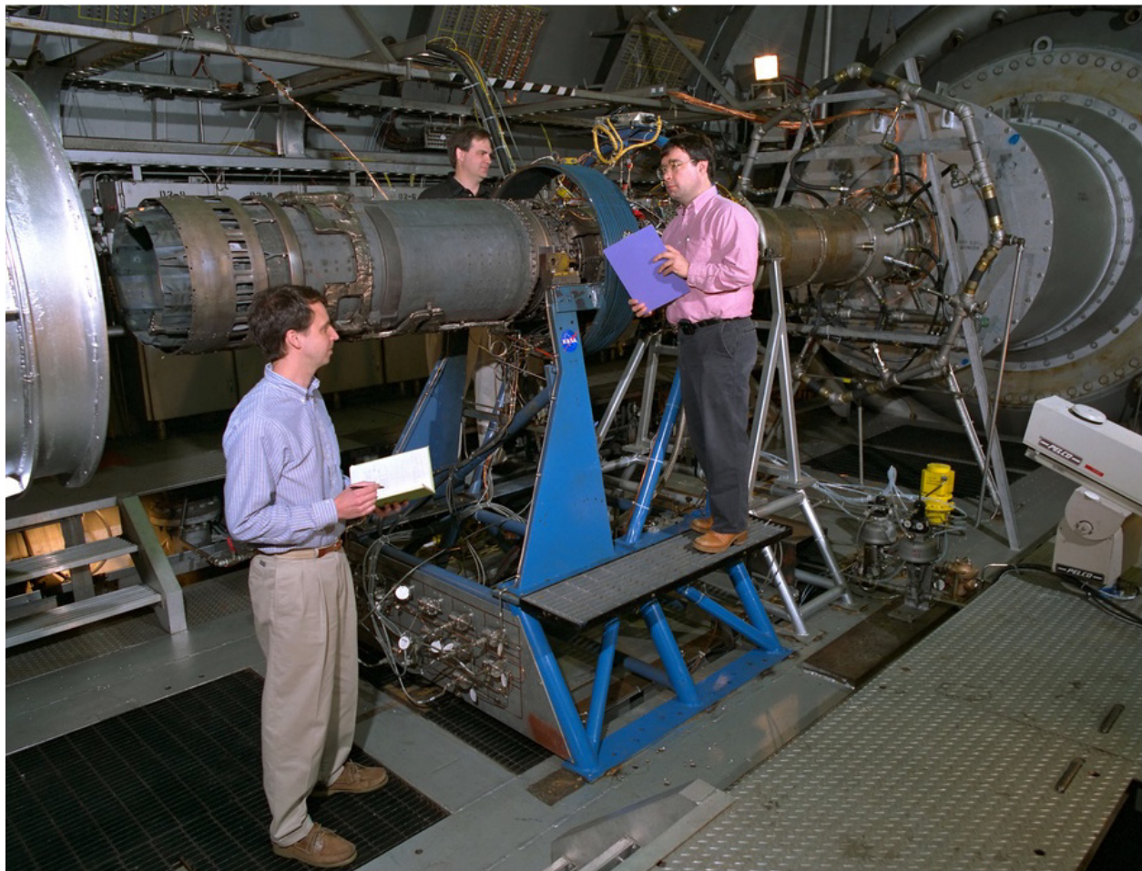
Figure 40.—High-altitude/high-speed engine test of General Electric J85 engine, 1998. (C-98-730)
