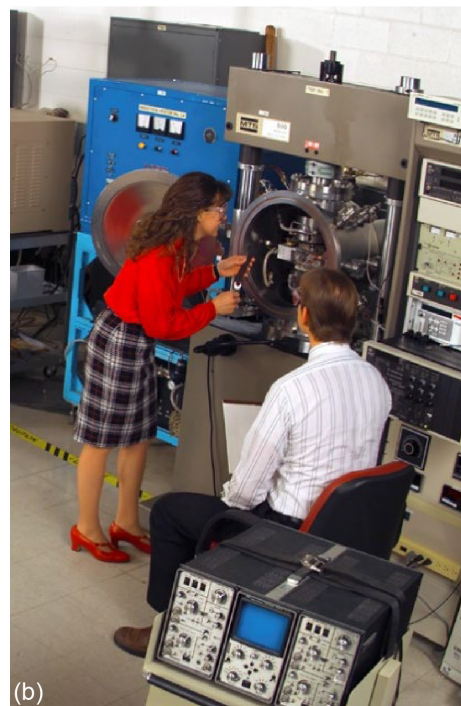
Figure 17.—Uniaxial electromechanical and servohydraulic test frames. (a) Instron® axial test rig with furnace oven capable of 1,400 °C. (b) MTS® axial test rig with environmental chamber for vacuum or inert environment testing.
