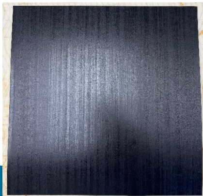
One ply of T1100/3960 prepreg.
