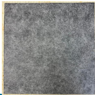
TPU veil added in between each ply.
