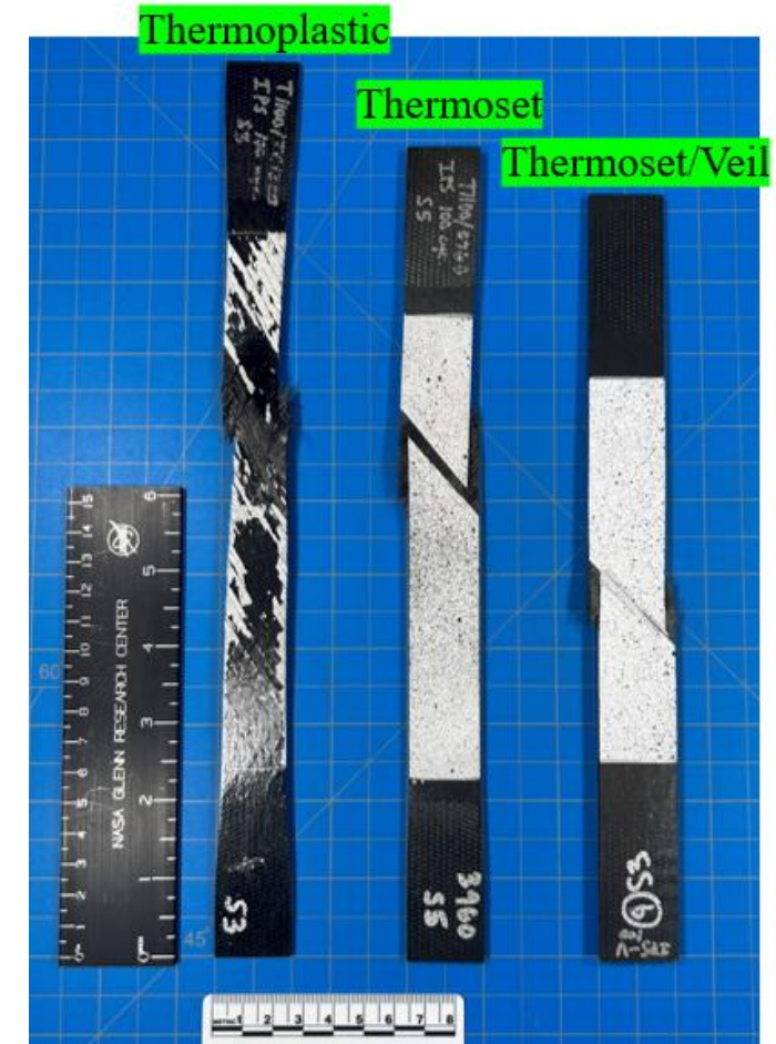
Failed IPS LN2-cycled coupons.
