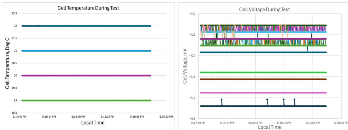
Figure 27. BMU data at impact. Cell temperature (left), and voltage (right)
