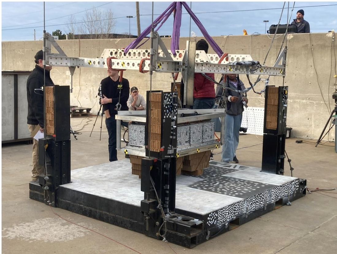
Figure 7. Bowtie marker positions on guided drop trolley and ESS hardware
