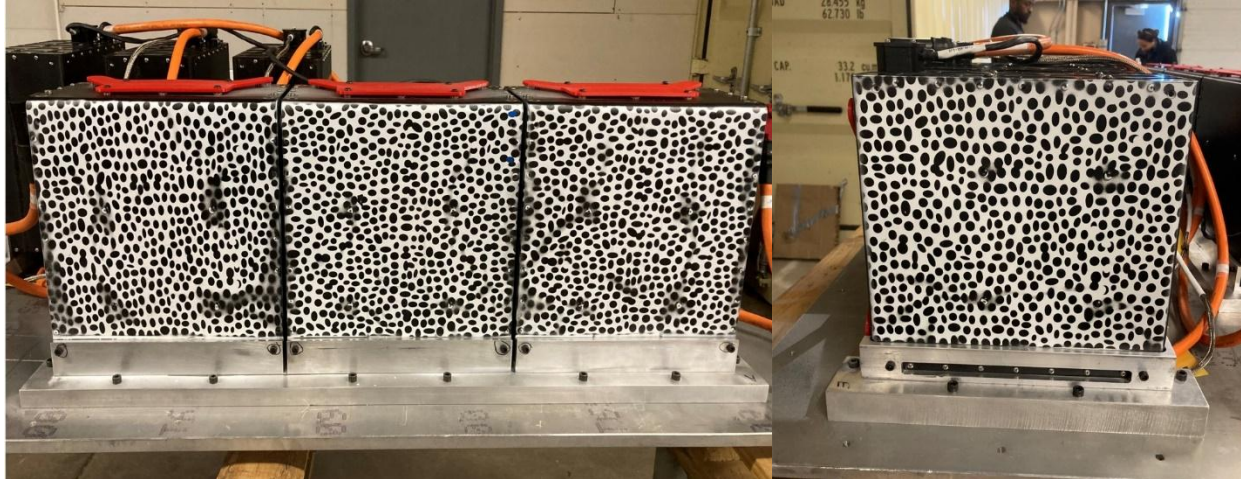
Figure 6. Speckle pattern on battery modules for 3D-DIC. Rightside Up (Left) and Sideways (Right)
