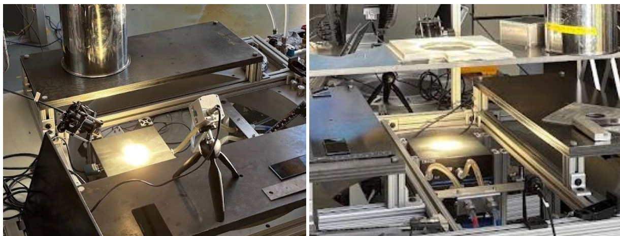
Figure 13: Calorimeter Test without Splash Plate (left) and with Splash Plate (right)
