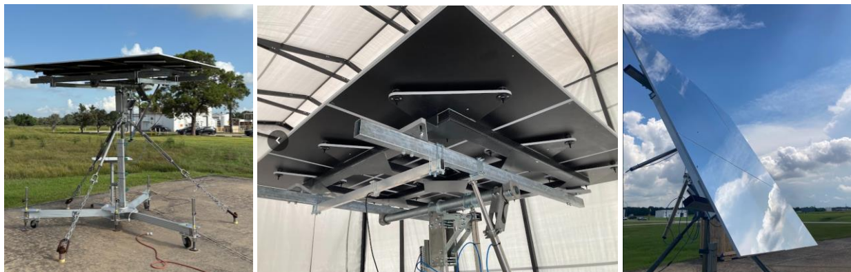
Figure 9: Complete Heliostat Assembly (left), Stowed in Tent (middle) and Tracking (right)
