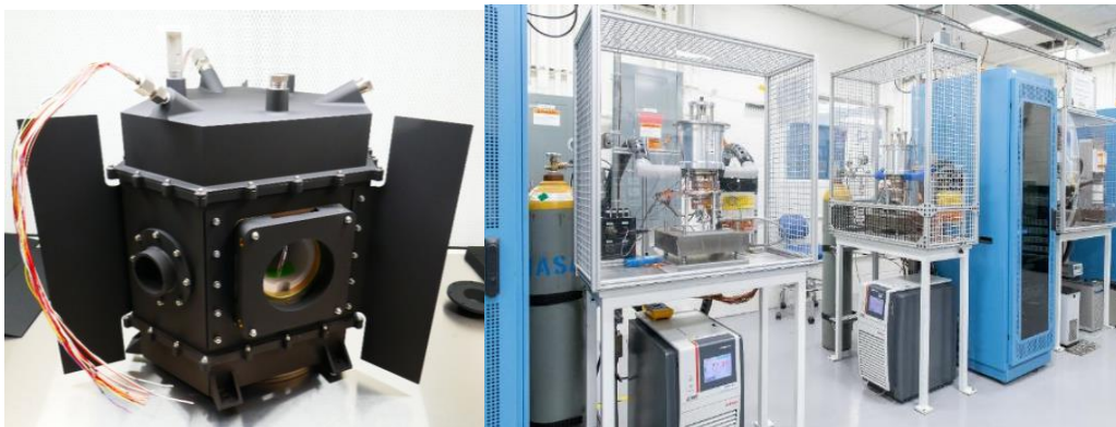
Figure 5-1: Left: Assembled electrically-heated heat source and housing at the University of Leicester. Right: SRL facility at NASA Glenn
