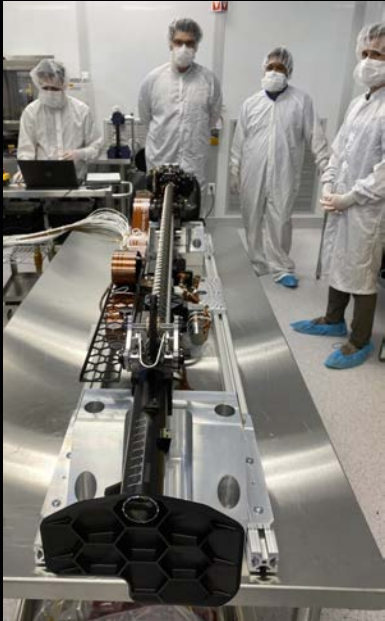
Subsurface excavation TRIDENT Drill
