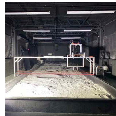
Sliding gantry over LHS-1 terrain
