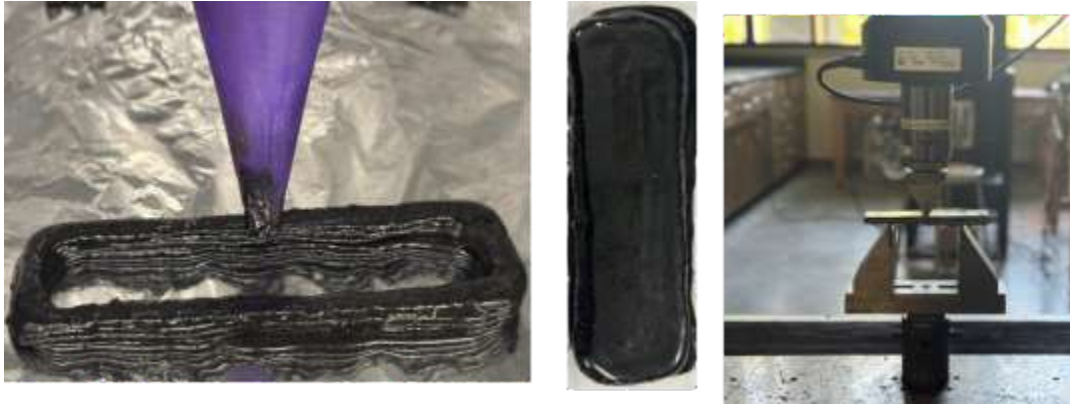
Figure 2. 3D Printing of Horizontal Sample and Printed Sample under 3-Point Bending Test
