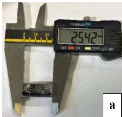
Figure 13. (a) The initial height of the specimen, (b) the height of the specimen after free shape recovery
