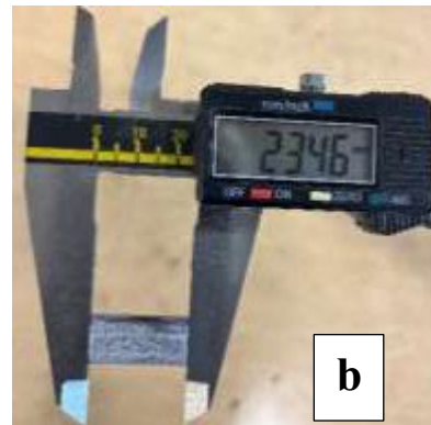
Figure 13. (a) The initial height of the specimen, (b) the height of the specimen after free shape recovery
