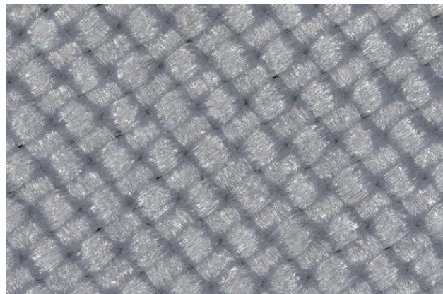
Figure 4. Calendared Teflon™ T-162 Fabric. At 50x, weave appears tighter with closed interstices.
