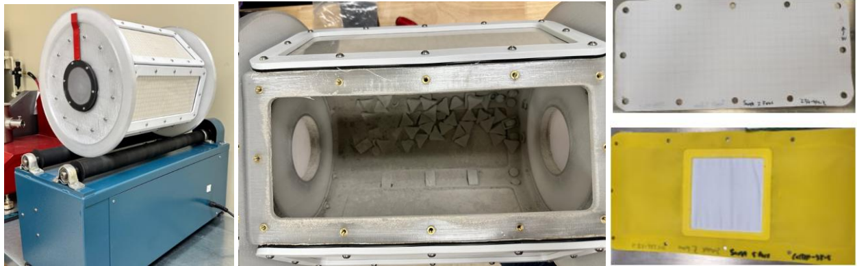
Figure 5. Rotary Abrasion Tumbler. (Left) Exterior of tumbler drum and roller base. (Center) Interior of drum showing lunar dust simulant and ceramic media. (Right top) A full panel of Ortho Fabric (Right bottom) Teflon™ T-162 fitted to a urethane coated nylon support frame.
