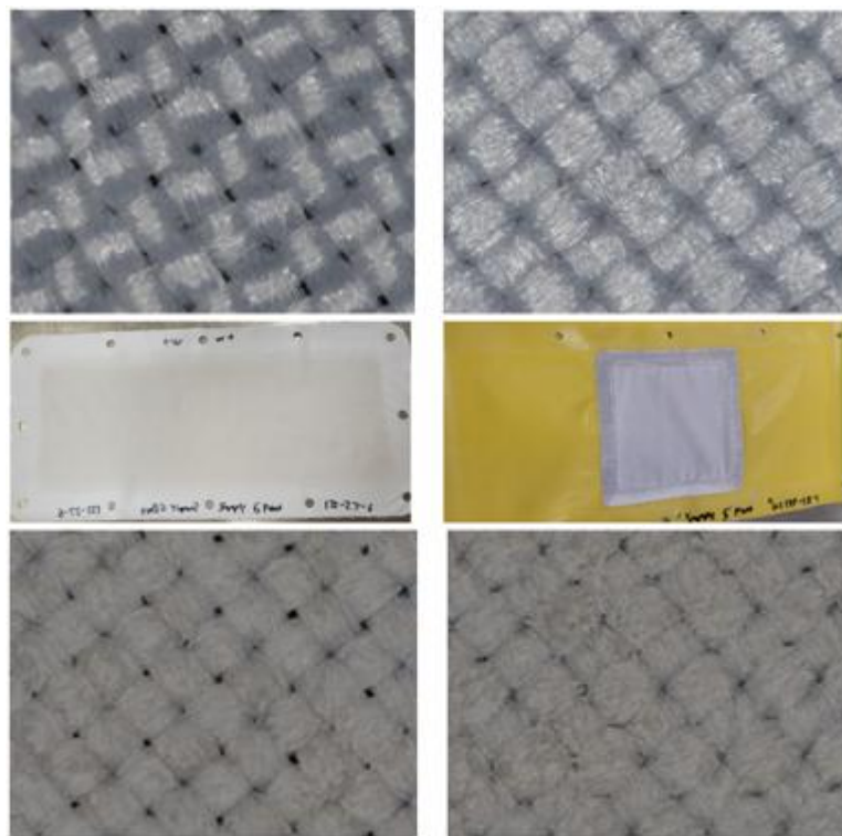
Figure 7. Teflon™ T-162 Tumbler Results. (Top Left) 100x Neat Teflon™ (Top Right) 100x Calendared Teflon™ (Center Left) Neat Teflon™ panel post tumbler and cleaning (Center Right) Calendared Teflon™ panel post tumbler and cleaning (Bottom Left) 100x Post tumbler neat Teflon™ (Bottom Right) 100x Post tumbler calendared Teflon™.
