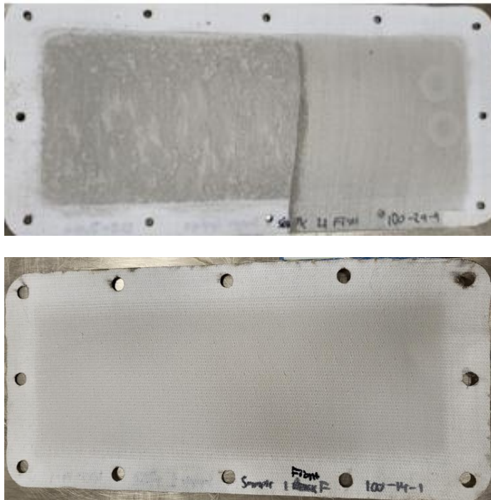
Figure 3. Ortho Panels Post Tumbler Dust Exposure. (Top) Left half covered with dust simulant, right half brushed. (Bottom) Post vacuuming.
