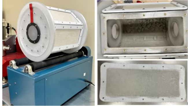
Figure 2. Rotary Abrasion Tumbler. (Left) Exterior of tumbler drum and roller base. (Right top) Interior of drum showing lunar dust simulant and ceramic media. (Right bottom) A full panel of dust covered Ortho Fabric.
