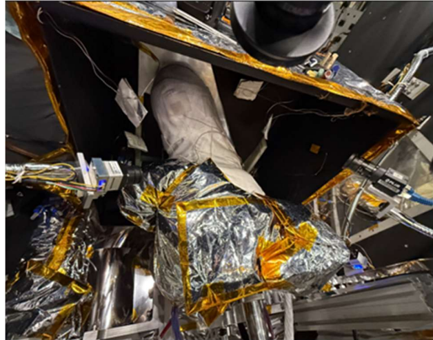
Figure 13: Spacesuit Boot Inside Mini-Shroud.
