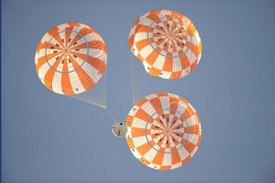
Orion CPAS Drop Testing
