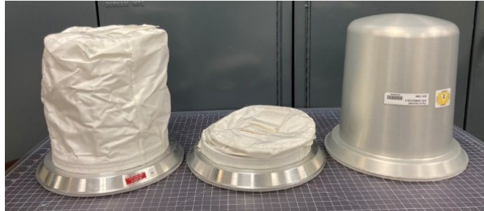
Figure 2. AFC in full configuration, empty (stowed) configuration and Hard-sided Canister.
