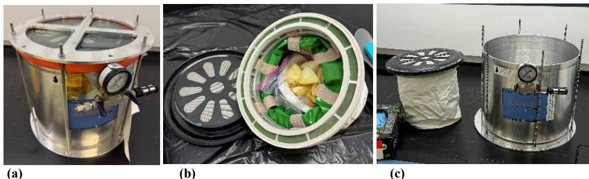
Figure 14. HFC gasket testing in small chamber (a) Top view, (b) AFC opened upon onion test conclusion (c) chamber opened under Hab Lab fume hood for fecal testing.
