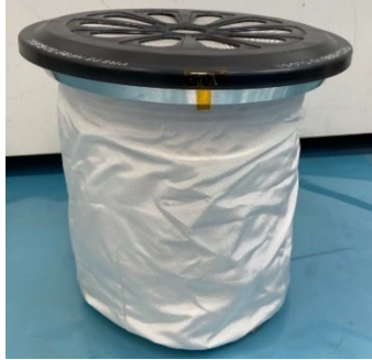
Figure 9. AFC filled for initial odor testing at WSTF.
