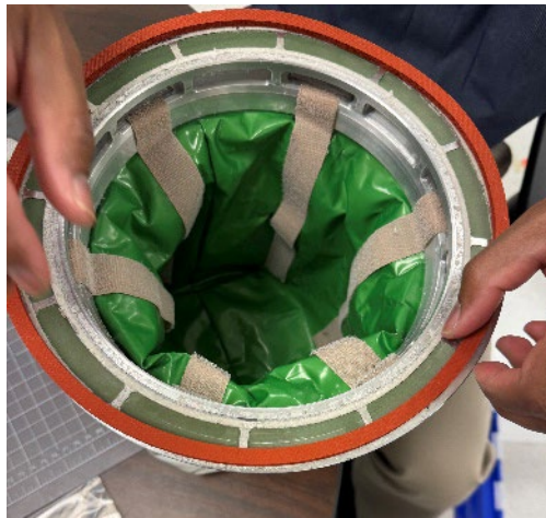
Figure 11. Gasket Images (a) Thinnest gasket candidate (1/8" thick HT-1240 solid silicone gasket) being applied to the AFC assembly.
