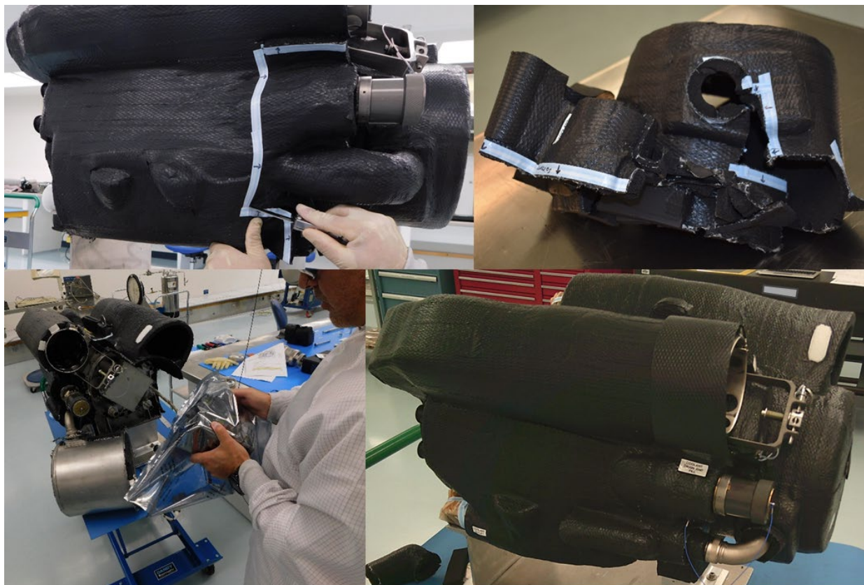
Figure 10: PPA Insulation Removal (Top), PFMC Removal (Bottom Left), and PPA Repaired (Bottom Right)
