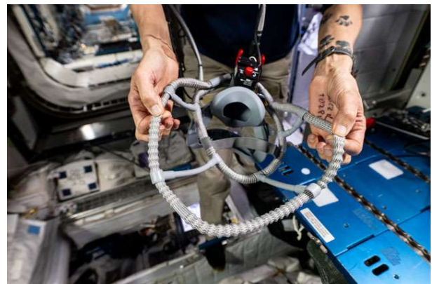
Figure 1. PHA QDMA S/N 1103 Ruptured Harness
