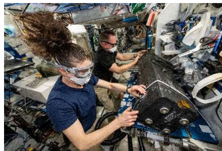
Figure 3. On-Orbit CDRA Bed Cleaning
