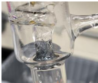
Figure A1. Crystallized Iodine at the Inlet of The Reflux Condenser.
