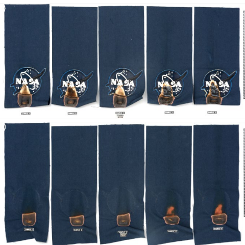
Figure 5. Custom fire-resistant patches sewn to crew clothing outer jacket fabric at 37% O 2 and 8.2 psia.
