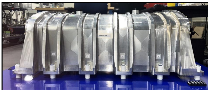
Figure 3. Mezzo Heat Exchanger, Starboard Side
