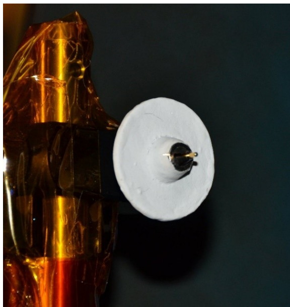
Figure 4. Custom-built reference target for in-situ laser alignment 19 .
