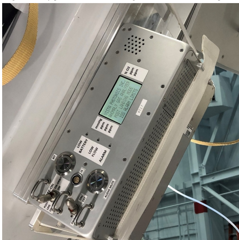
Figure 4. AGA EDU. The 9-gas EDU included a hydrazine channel that was ultimately removed in the flight units. The flight version also has much more substantial mounting of the unit to the Orion bulkhead. The unit is shown running in the Orion mock-up at NASA JSC.
