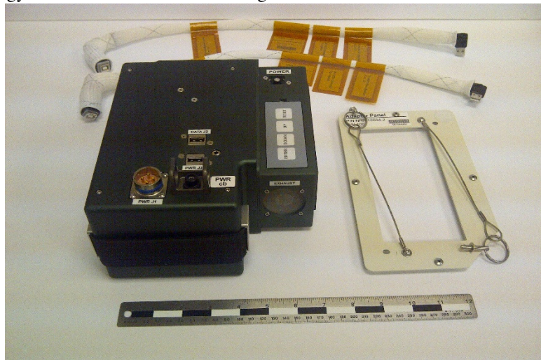
Figure 1. Sensor version 4.0, Multi-Gas Monitor. Flight prototype version 4.0 after assembly and integration. The adaptor plate allows for mounting to ISS equipment racks. The sensor can be powered through two USB ports or 28 VDC rack power.
