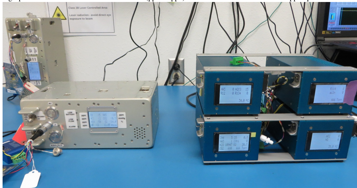
Figure 8. AGA and submarine AGA. The flight certified AGA is shown beside the submarine AGA prototype. The submarine AGA is comprised of four modules. Three of the modules are dedicated PAS and provide ppb to ppm level detection of multiple gases. Data is logged independently by each module as well as streamed over an RS-485 interface. The submarine AGA weighs about 10 kg.
