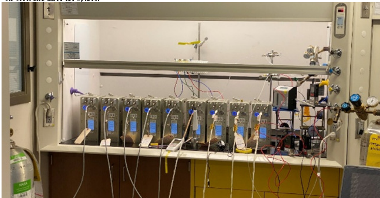
Figure 5. AGA Calibration. AGA calibration is a several week activity given the variation in gases, concentrations and environmental conditions required to characterize the AGA response behavior. However, most of the time is spent in setting up the blended gas. It is not much more difficult to calibrated multiple AGAs point-by-point sequentially. Nine AGAs were calibrated during the last campaign.
