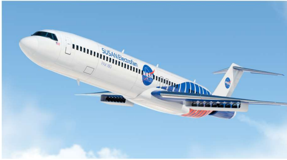
Figure 6. SUSAN showing the 16 wingfans in a mail slot configuration under the wings.
