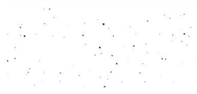
G20-P80 Segmented X-ray CT Image, Porosity 1.00%
