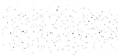
G25-P75 Segmented X-ray CT Image, Porosity 3.18%
