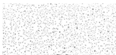
G50-P50 Segmented X-ray CT Image, Porosity 7.91%
