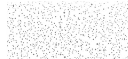
G70-P30 Segmented X-ray CT Image, Porosity 7.48%
