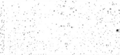
G100-P0 Segmented X-ray CT Image, Porosity 2.51%
