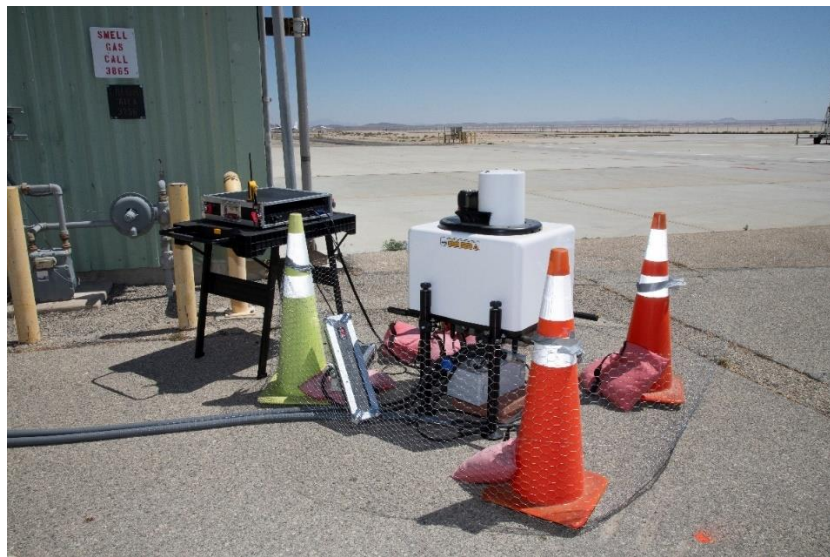
Figure 2. One of two, Doppler wind lidars near the hangar at AFRC
