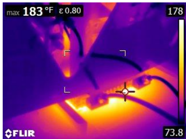
Bladder during welding
