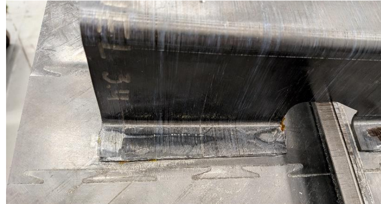
Overheating of shear tie & skin ply squeeze out
