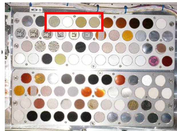
(Left) MISSE-8 samples mounted outside the International Space Station. (Right) MISSE-8 material samples with the materials described here in the red box.
