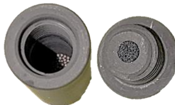
Figure 2: Sample Holder Designed for 1g of TRISO Fuel Particles
