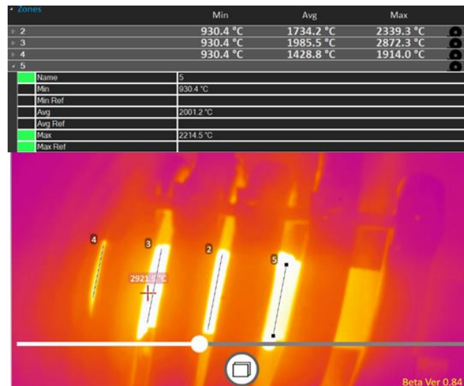
Figure 10: Side IR Camera Capture During TSR-01 Testing within NTREES
