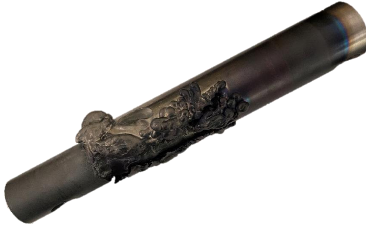
Figure 11: Partially Deconstructed TSR-01 Post-Test with Melted Tungsten Outer Sleeve
