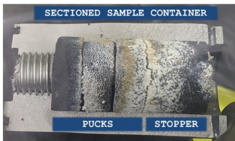
Figure 17: Sectioned Sample Volume Assembly
