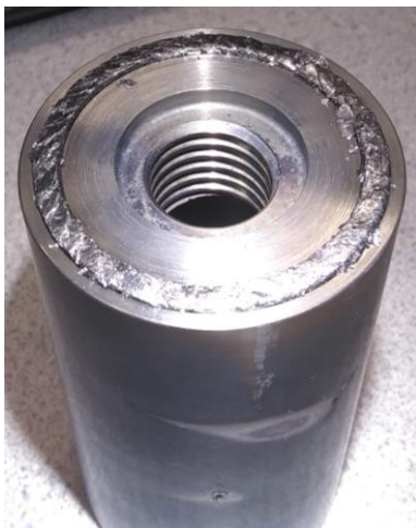
Figure 8: Sample Container with Graphite Packing
