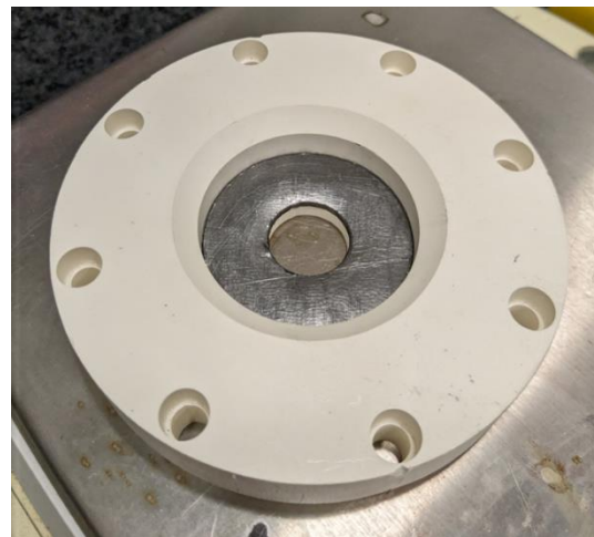
Figure 9: Hot Clamp Interface with Addition of Graphite Gasket
