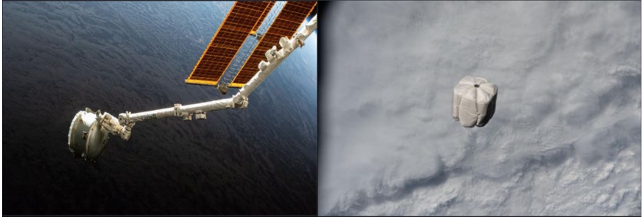
Fig. 9 Released images from the first trash deploy from the Nanoracks Airlock: Left - Nanoracks Airlock on a robotic arm [6]; Right - Trash container after being jettisoned from the Nanoracks Airlock [7].
