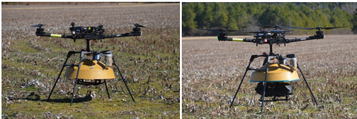
Fig. 5 Subscale drop test article mounted to an Alta X carrier drone in the stowed configuration (left) and in the posed configuration (right).
