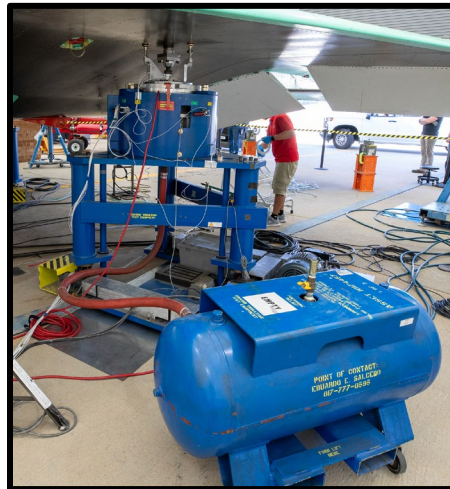
Figure 12: Soft support system installed at left- aft jack point.
