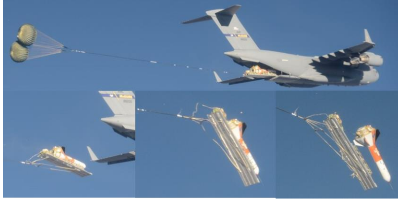
Figure 6. Mated vehicle extraction through programmer line stretch
