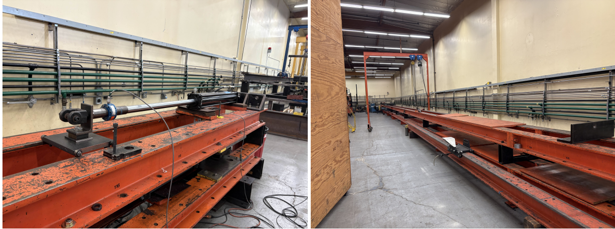
Fig. 2 Large tensile test stand for testing of full-scale elastic elements at Tension Member Technologies (TMT) Laboratories in Huntington Beach, CA. Hydraulic driver with 40-kip load cell (left) and full 110-ft test segment available for use (right).
