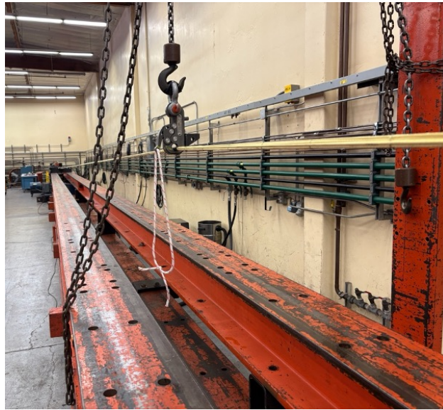
Fig. 9 Flight-like riser mounted to the horizontal test stand. The gantry crane with quick release hook is attached at the center of the specimen.
