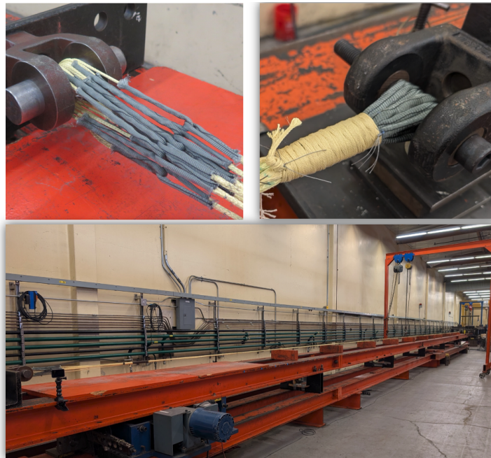
Fig. 7 Flight-like riser mounted to the test stand for static cycle testing. Full test setup (bottom) with close-ups of the dead end side continuous loop attachment (top left) and the hydraulic side pin attachment (top right).
