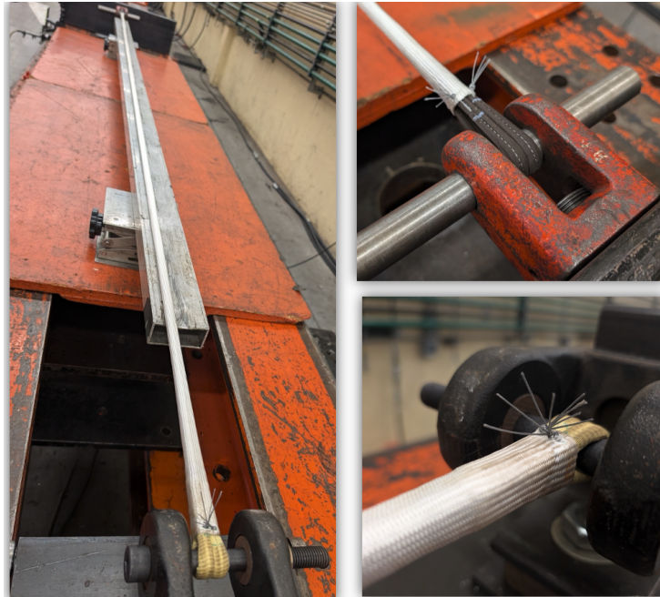
Fig. 6 Flight-like bridle mounted to the test stand for static cycle testing. Full test setup (left) with close-ups of the dead end side pin attachment (top right) and the hydraulic side pin attachment (bottom right).
