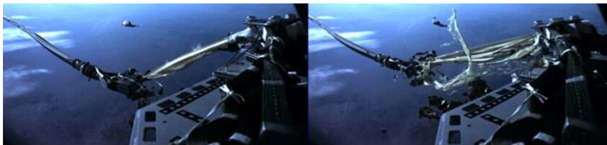
Figure 4. CDT 3-16 Reposition Deployment Line Damage
