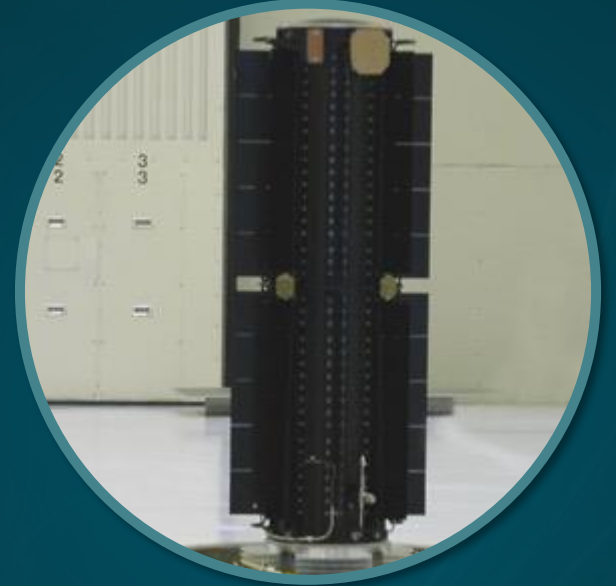
Vacuum-Rated Radioisotope Power System
