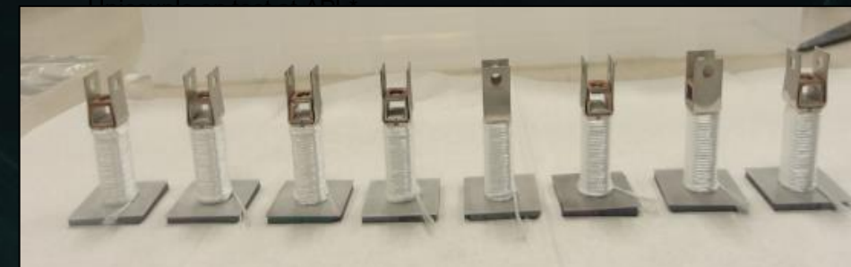
New Material SiGe Unicouples Produced at TESI
