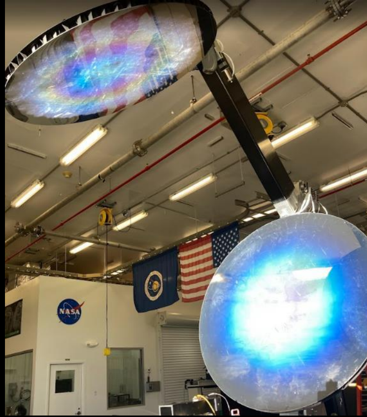
Heliostat and Tracking (Left), Illuminated Solar Concentrator (Middle) and Molten JSC-1A Simulant at Focal Point (Right)
