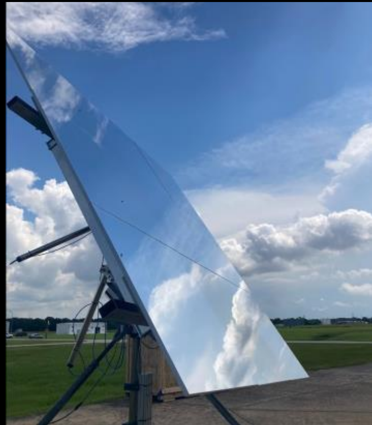
Heliostat and Tracking (Left), Illuminated Solar Concentrator (Middle) and Molten JSC-1A Simulant at Focal Point (Right)
