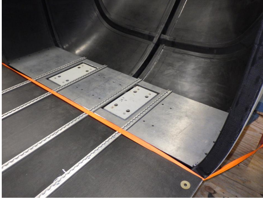
Figure 5. ESS mounting fixture and ballast mass
