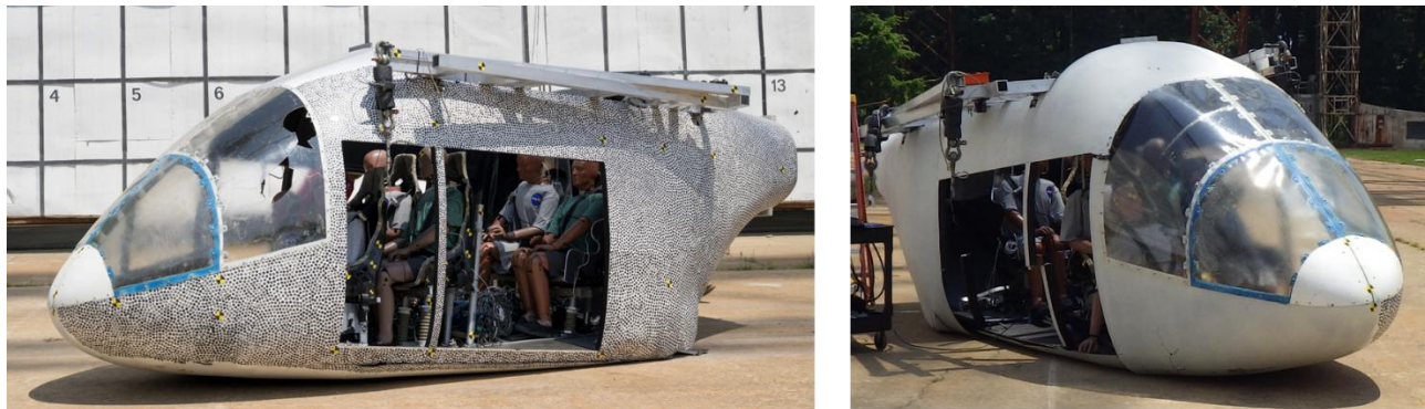
Figure 16. Post-test configuration of the test article. Port side (left) and Starboard side (right)
