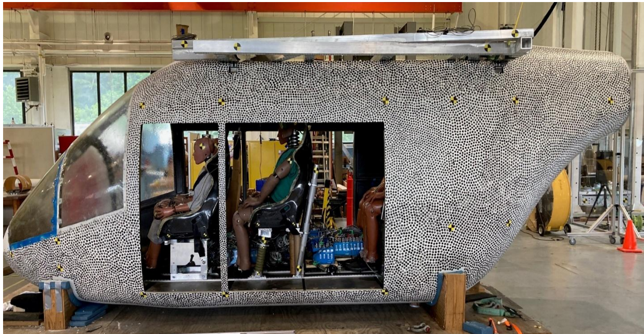
Figure 11. Speckle pattern on port-side of vehicle for 3D-DIC
