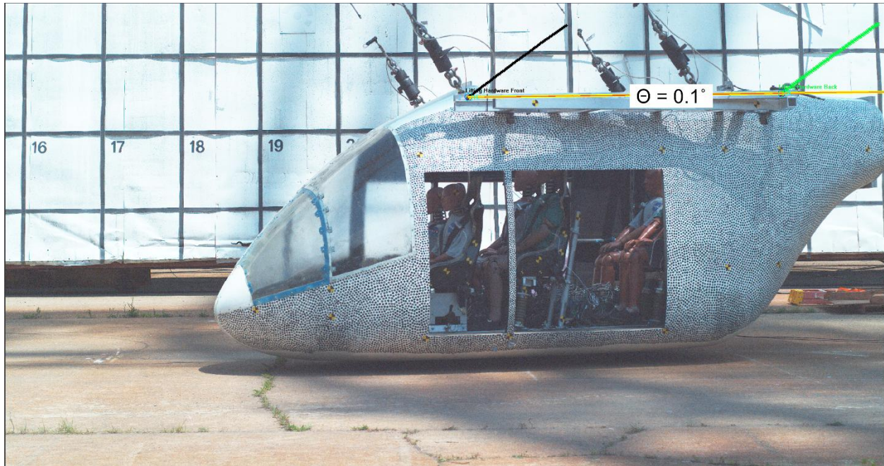
Figure 26. South (port-side) view showing pitch angle at impact
