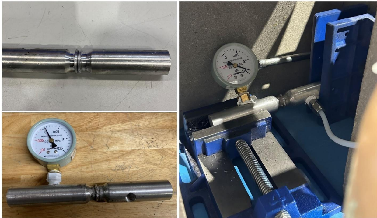
Figure 2.5.1: The final flanged pipe design used for PE3D pipe section fusion joints (top left). Welded pipe segments integrated with pressure gage (bottom left), pressure test to 20 psig (right). The pipe material is aluminum 6061 with a 1-inch outside diameter.
