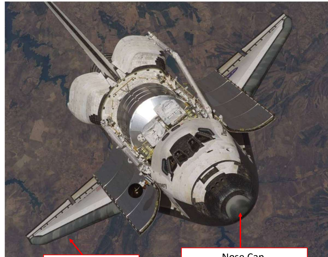
Wing Leading Edge Panels and Seals
