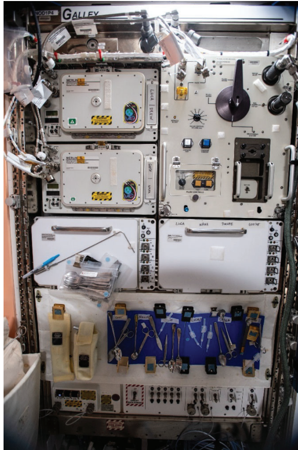
Figure 23. ISS Galley Rack Prior to Late 2020 Contains two cold-storage MERLIN lockers (stacked top left), the PWD (top right), two Galley food warmers (side-by-side below MERLIN and PWD), and storage (bottom).
