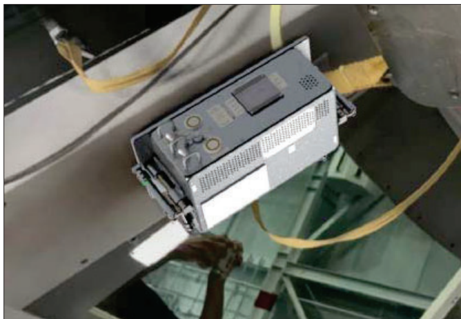
Figure 15. Anomaly Gas Analyzer Mounted in MPCV CM
