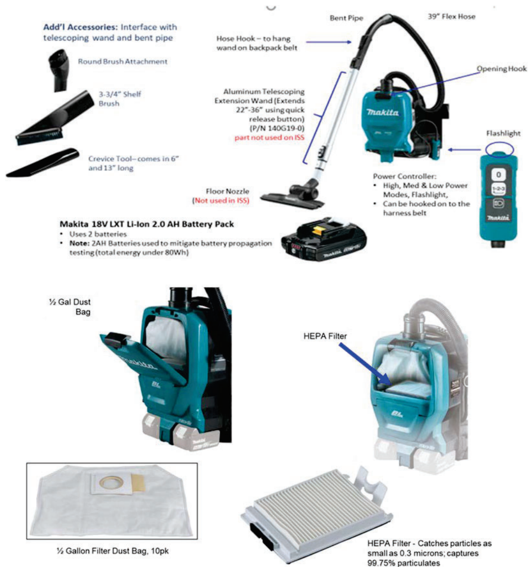
Figure 21. Makita Vacuum Components
